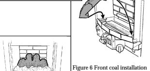
Place the rear base coal in the burner compartment behind the front coal. It should rest on the ledge at the back of the burner compartment and its rear face should touch the rear ceramic wall (See figure 7).
